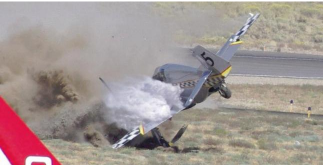
High octane aviation fuel spewed from the left wing as the engine separated from the
