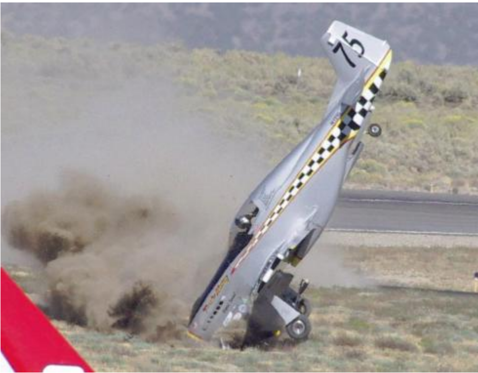
The wing tip dug into the sand and the aircraft cart wheeled.
